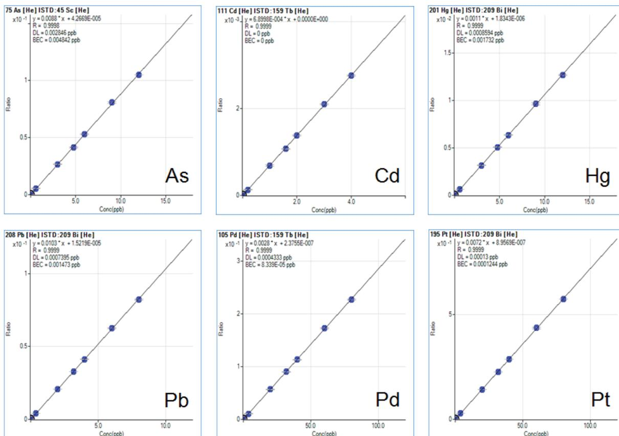
**Figure 1.** Calibrations for As, Cd, Hg, Pb, Pd and Pt in He mode, demonstrating limits of detection of 1 ng/L or below, and good sensitivity and linearity for all elements including Hg, Pd and Pt, which require stabilization in HCl
