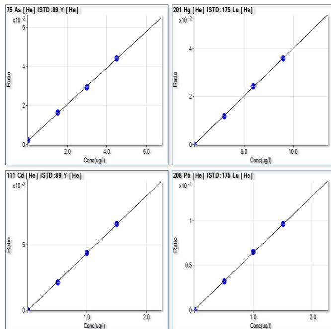
**Figure 2.** Calibration graphs for As, Cd, Hg, and Pb.
