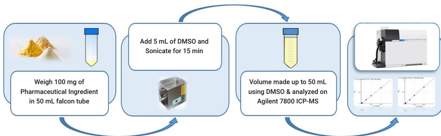
**Figure 1.** Flow diagram for sample preparation and analysis using the Agilent ICP-MS.
