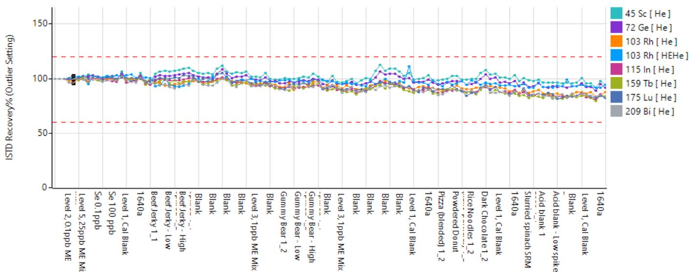
Figure 3. Stability of ISTD measurements over 12 hours. The ISTD recoveries have been normalized to the calibration blank for all samples.
