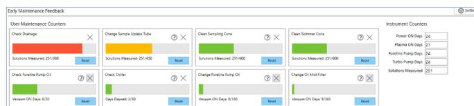
Figure 3. To maintain peak ICP-MS performance, EMF prompts maintenance such as cleaning the interface cones, adjusting or replacing the pump tubing, etc. after a specified number of samples have been analyzed.
