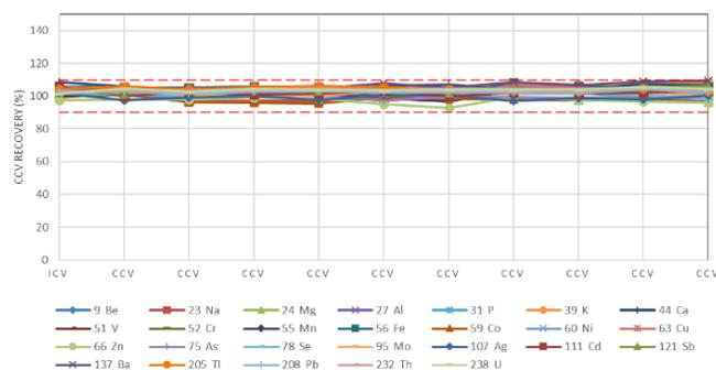
Figure 2. CCV stability over the eight hour sequence. All CCV recoveries were within 10%.
