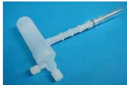
**Figure 9.** Inert (HF resistant) O-ring-free PFA sample introduction system.
