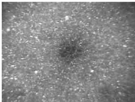
**Figure 5.** CCD image of the BaTiO<sub>3</sub> disk after laser irradiation showing minimal damage (laser diameter was 10 μm).
