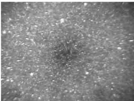
**Figure 4.** CCD image of the BaTiO<sub>3</sub> disk prior to laser irradiation.
