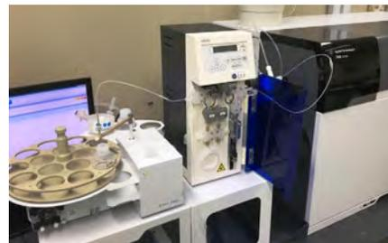
**Figure 12.** The ASAS automated standard addition device, part of the CSI online monitoring system from IAS Inc., Japan.
