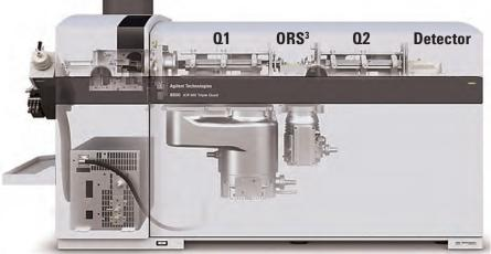
Figure 1. Cutaway diagram of the Agilent 8800 ICP-000
