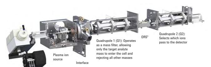
Figure 1. Schematic of the Agilent 8800 Triple Quadrupole ICP-MS
